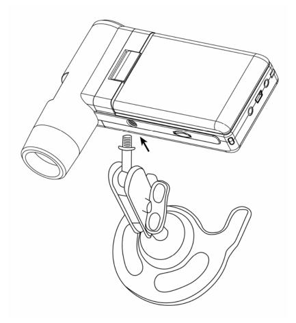
Do not force the end into the hole; forcing may damage the microscope.
