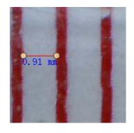
2) Multi-line: click , left-click mouse to choose a start point and drag to an end point. Notice that the measurements are displayed as you go along. Release mouse when done. You can continue measuring from the previous end point to a next point and so on.
