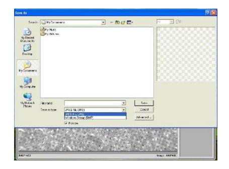
The file can be saved in either jpeg or bmp. The jpeg size in which the photo is saved is the maximum allowed for jpeg. You can choose to decrease the size by adjusting quality. Click the Advanced button to view and select jpeg save options.
