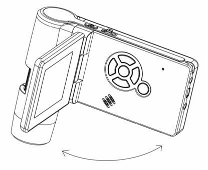
2) If need to power on when panel unfolded, press POWER ON/OFF button.
