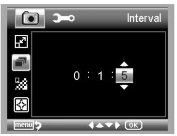
**Interval:** input interval time between frame capture by UP/DOWN and LEFT/RIGHT.
