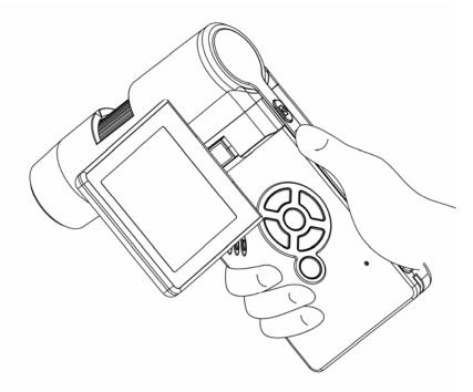
4) When a clear image got, hold the microscope steadily and press Capture button (1) one time.
