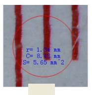
4) Circle-diameter: click S, left-clicking to choose a start point for a circle; draw the circle to an end point, release the mouse, and the radius of the circle will be displayed.
