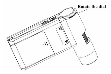
3) Hold the microscope main body by right hand; put the viewing end closely to target object; adjust focus wheel to get clear image by left hand.
